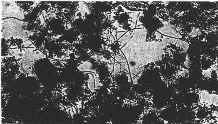
As bulking progresses, protozoa become less noticeable and filamentous growth becomes apparent. This is the state at which treatment with hydrogen peroxide should begin
